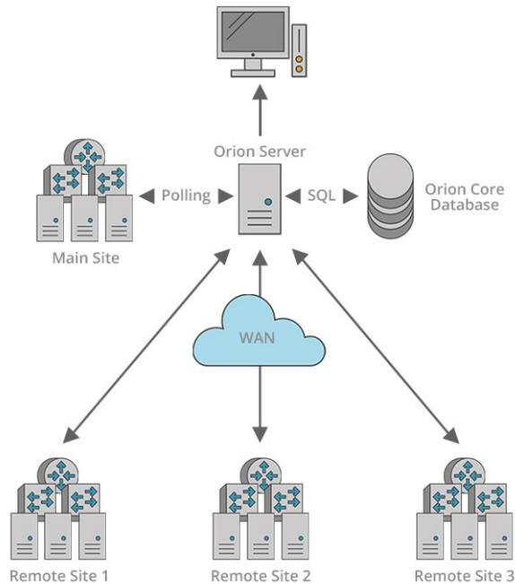
A reliable static connection is required between the primary region and all monitoring regions. This connection is continually transmitting monitoring data. The quantity of bandwidth consumed will depend on many factors, including the type and number of SolarWinds Orion Platform products that are installed, and the types and quantity of monitored elements.
