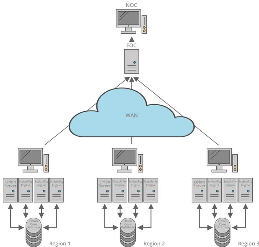
SolarWinds EOC securely collects Orion Platform-based server data directly from each of the regional Orion servers. WAN performance is not impacted because Orion servers poll network devices locally and EOC only periodically pulls updates from each Orion Platform-based server database.
