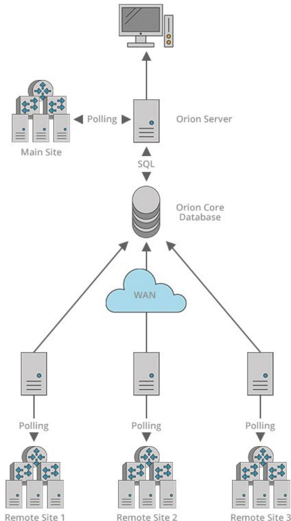
Scalability engines poll data locally in each region, and the polled data is then stored centrally on the Orion database server in the primary region. Regional operators in each region log into the Orion web console in the primary region where the Orion Platform is installed to view data.
